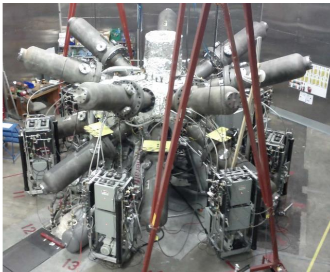
Fig. 4. Mini-Sphere: a 1 meter spherical vessel filled with liquid lead with a synchronized array of 14 full-scale acoustic drivers mounted around the exterior, arranged in two rings of 7 drivers each. The hammers impact anvils that are in direct contact with the liquid lead, imparting pressure pulses into the molten metal. Lead is pumped around the inside of the sphere, creating a cylindrical vortex in the centre of the device. The inner wall of the vortex can then be imaged with fast cameras to record the collapse dynamics.
