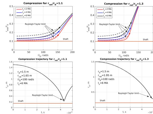
Figure 3: Rayleigh-Taylor stability limits and no-plasma compression trajectories.
