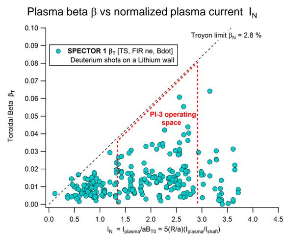
**SPECTOR** achieved its best performance in terms of temperature, overall magnetic lifetime, and plasma stability at a relatively low- $\beta$  range, 1- 5% , bounded by the empirical Troyon limit for Ohmically heated tokamaks, which is reasonable considering SPECTOR's lack of additional heating.
