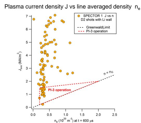
**SPECTOR** typically operated in the low-density edge of parameter space, just at the boundary of the run-way limit, confirmed by the detection of hard X-ray emission from a significant population of run-away electrons. High performance shots routinely achieved high temperature operation over a wide range of total plasma current.
