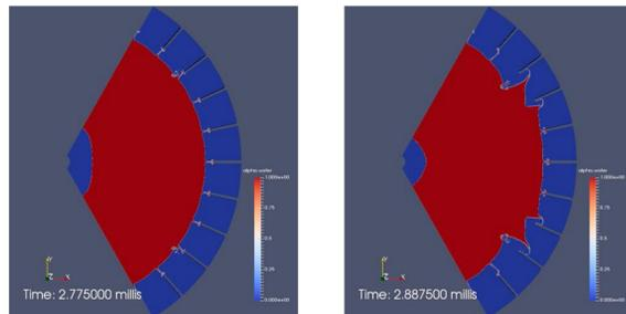
Above (left) cross-section shows a compressed, elongated cavity from equal pressure drive pressure, where above (right) shows a more self-similar compressed cavity geometry when the drive pressure is reduced towards the equator. By adhering to, or deviating from, a self-similar compression, the compression geometry can be optimized for plasma stability.
