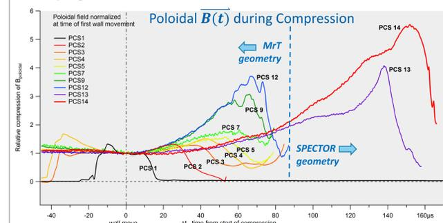
Once radiation was eliminated as the dominant energy loss during compression after PCS7, MHD stability during compression was the limit. The addition of shaft current on PCS12 and better compression geometry on PCS13 resulted in the next big improvements.
