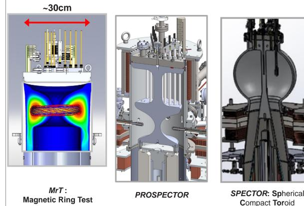
**Spheromak Plasmas ( $q < 1$ ):** Large improvements in magnetic and thermal lifetime were made on the **MrT** style single-stage injectors. The greatest improvement came by modifying the global  $q$  profile by maintaining small amounts of poloidal gun current after the main formation pulse to avoid radial surfaces and to "sustain" plasma life.
