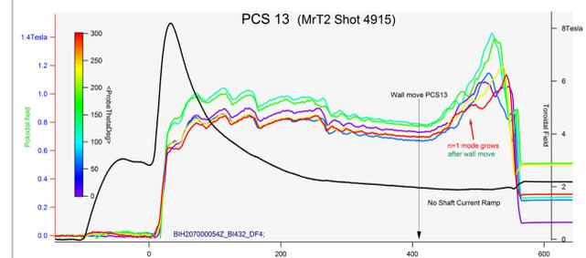
Further improvement of MHD stability was achieved on PCS14 by ramping the shaft current during wall move such that it roughly balances the increase in plasma current.
