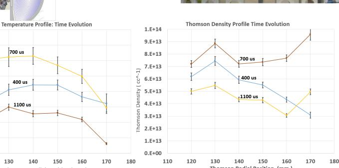
The temperatures and thermal confinement times of these plasmas are within the range needed to be considered as targets for adiabatic compression to fusion conditions. Our plasma development can now have increased focus on performance of our CTs under compression. We are addressing this issue through a combination of simulation and experiment.
