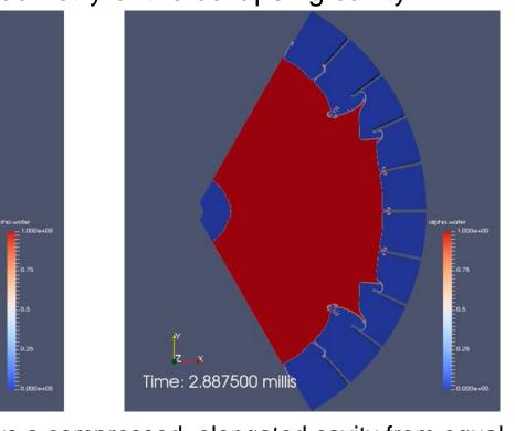
Above (left) cross-section shows a compressed, elongated cavity from equal pressure drive pressure, where above (right) shows a more self-similar compressed cavity geometry when the drive pressure is reduced towards the equator. By adhering to, or deviating from, a self-similar compression, the compression geometry can be optimized for plasma stability.
