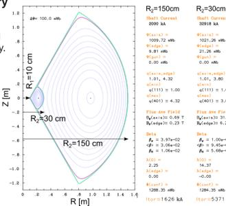
In leftmost column are initial equilibria varying by shaft current. The plasma pressure and current profiles are all the same.
