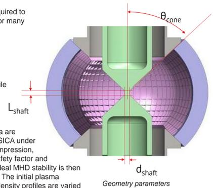
Sequences of equilibria are generated using CORSICA under ideal and adiabatic compression, conserving both the safety factor and entropy profiles. The ideal MHD stability is then computed with DCON. The initial plasma pressure and current density profiles are varied to optimize the stability boundaries.
