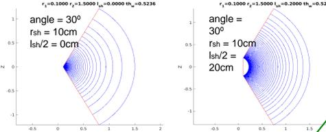
Geometry affects the stability primarily by altering the  $q$  profile. The longer shaft reduces the  $q$  profile for a given initial shaft current.
