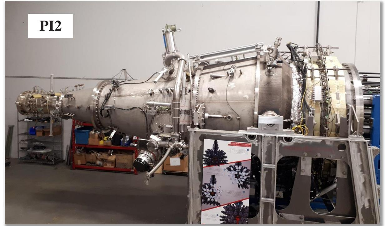
The accelerating railgun electrodes were conically converging to achieve the 4x radial compression to bridge the gap between the densities achievable with Marshall gun formation, and what was required for the initial state of the proposed MTF compression scenario.
