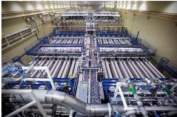
Figure 12. Photo of 1.8MJ laser bay of the National Ignition Facility at Lawrence Livermore National Laboratory.
