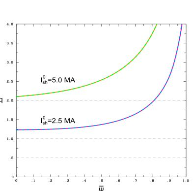
• On the left is the pressure profile for two starting shaft currents. Each case starts with the same profile, but flux surfaces compress differently, so final profiles are different. Adiabatic compression goes as P<sup>5</sup>, but most compression is near the core, so peak pressure increases faster.  $(5000 > 5^5 = 3125).$
