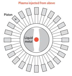
Plasma is compressed by the liquid-metal lining of the reaction chamber, itself pushed inward by pistons
