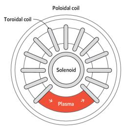
Plasma fuel is confined and heated by electromagnets arranged around a toroidal reaction chamber
