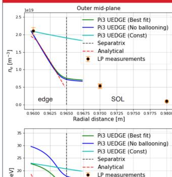
Plasma diffusion models can be developed by combining Langmuir radial scans with UEDGE plasma simulations.
