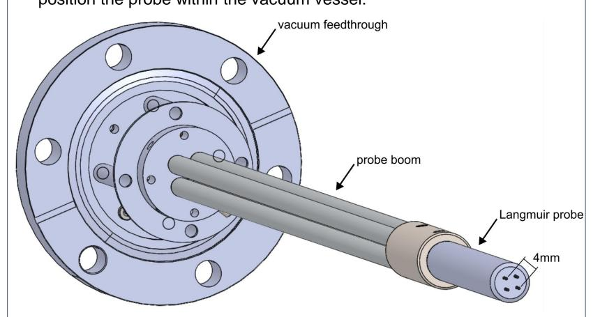
The probe boom and bellows system is dimensioned such that the probe can be protected behind a gate valve during lithium coating.
