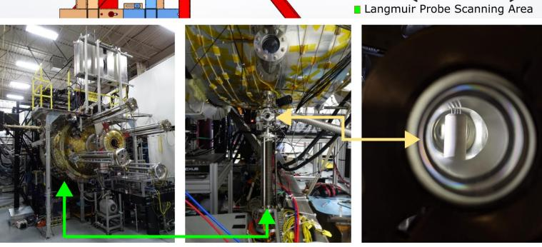
The probe's installation and operating region is illustrated above. The probe's depth is limited by the probe's ability to withstand plasma heat flux and its disturbance to the plasma.
