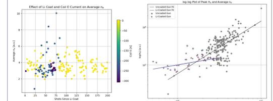
We also see that H<sub>α</sub> (656 nm) peak intensity decreases significantly after Li coating the gun, as observed with the survey spectrometer [a.u.]. However, the ratio of H<sub>α</sub>/n<sub>e</sub><sup>2</sup> increases significantly due to Li coating (by >73%), this could be caused by either an increase of plasma edge temperature, or a decrease of Z<sub>avg</sub>, both of which are plausible effects from Li gettingting.
