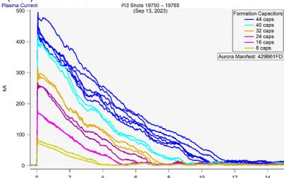
As the formation bank energy U<sub>form</sub> is increased by adding caps at constant voltage, the poloidal magnetic energy efficiency U<sub>pol</sub>/U<sub>form</sub> increases nearly linearly with bank energy in a favorable scaling for larger machines. These scans were repeated over 3 runs with differing amounts of initial toroidal field: Run 1, 3 at V<sub>peak</sub> = 7 kV, Run 2 at V<sub>peak</sub> = 4 kV, while Run 3 also had the shaft sustain circuit on at V<sub>sust</sub> = 7 kV.
