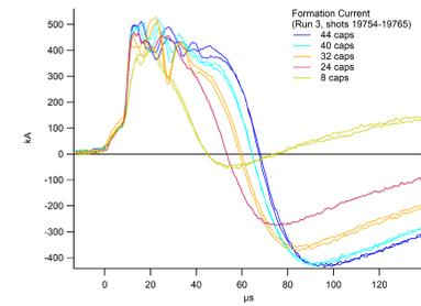
The peak of formation current is similar for all cases, and enough to always pass the ideal bubble-out threshold, however the pulse width almost doubles and the resulting increase in plasma current (5x) and total lifetime (2.5x) is dramatic.
