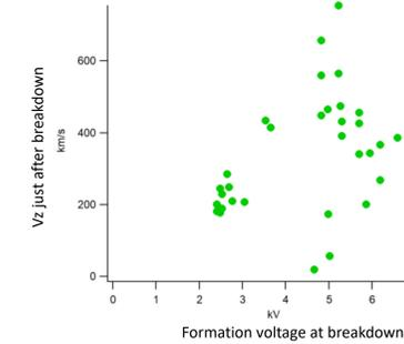
Increasing the plasma velocity during bubble-out corresponds to a higher initial ion kinetic energy, which will then thermalize over time to yield a higher ion temperature. It is desirable to begin the MTF compression with as high of ion temperature as possible, since the temperature gain factor is challenging to increase.
